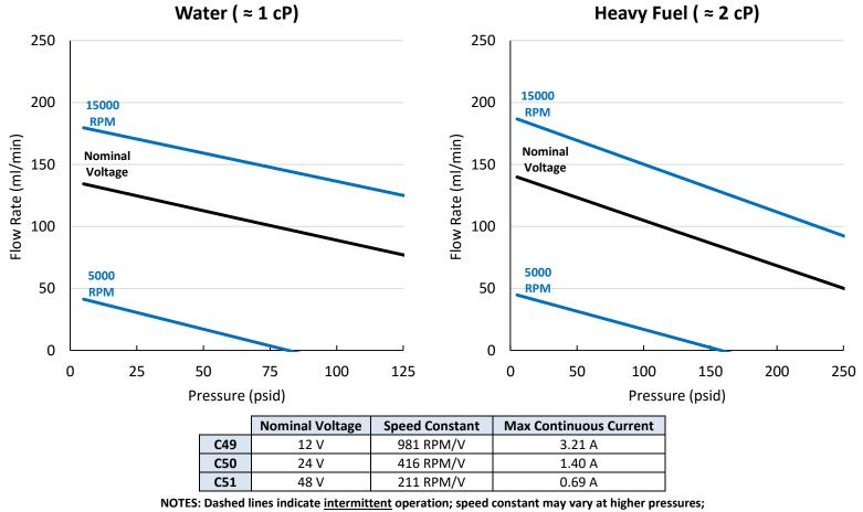
RPM flow lines indicate performance at typical maximum and minimum speeds;
